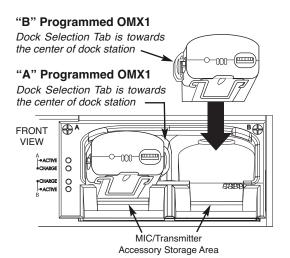
When storing the OMX1 MIC/Transmitter into the ORB35 Loading Dock for charging, insert it on a slight angle, with the front face of the OMX1 pointing up.
